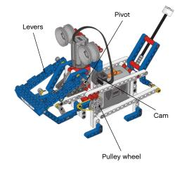
The jaw and tail movements both feature compound levers with several pivots.
