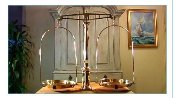
The simplest weighing machine is a beam balance. The original form of a balance consisted of a beam with a fulcrum at its center. A change of weigh on either side of the balance will change the beams positioning and effect the balance achieved.
