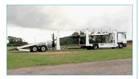
Ramps have been used since ancient times to help move heavy objects or large quantities of materials from one level to another. Today, automobile transport services use ramp on their trucks to load multiple vehicles on one transport. These multi-vehicle transports use ramps for easy of use, safety and efficiency.
